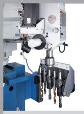
Automatic Tool Changing system (ATC) for 5 tools (Pos. 8.10) at the right side of the machine
