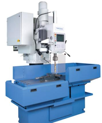
Splash and chip guard (Pos. 11.30), vertically movable, 2-piece unit. Either side can be moved down
